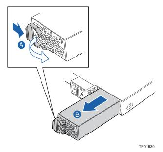
Figure 46. Removing the Rear Hot-Swap Power Supply from the Chassis
